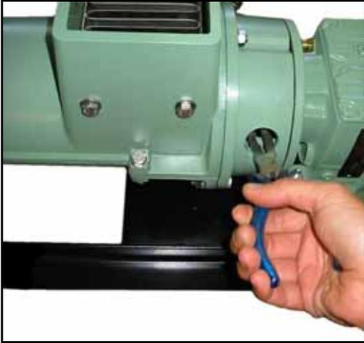
**Figure 2. Removing the Auger locking screw.**
