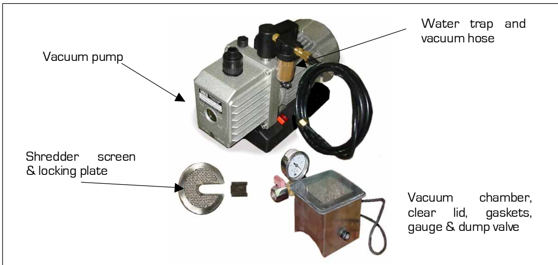
Figure 3: The vacuum module.
