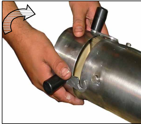
Figure 9: Fitting the Die Holder to the barrel
