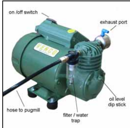
Figure 6: Vacuum hose and filter location on the vacuum pump
