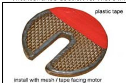
**Figure 4: Blanking off the shredder screen**
