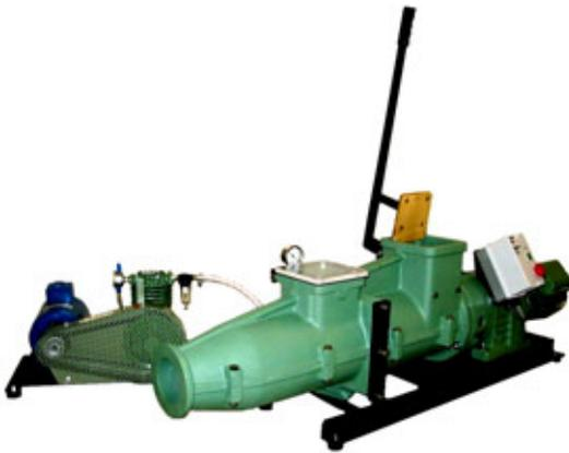
75mm, 87mm and 100mm (3 1/2, 4") single auger de-airing pugmill
