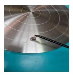
REPLACE BAT PINS WITH BLANKING PLUGS USING A 4MM ALLEN KEY.
